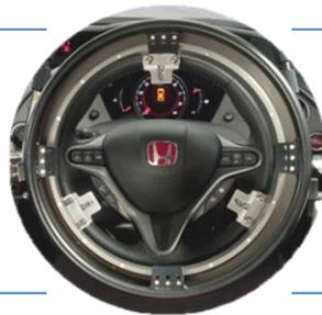
custom steering column adaptors. The main benefit, however, is seen in modern vehicles where the removal of the driver's airbag may be detected by the ESC system, triggering a change in the vehicle's dynamic limits. With the SR15 or the Torus, this problem is solved.
